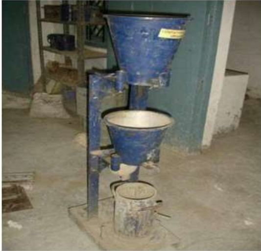
Figure 4.7: apparatus of compaction factor test
