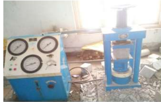
Figure 3.8: Compressive testing machine
